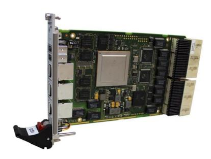
The G51 single-board computer unites the benefits of CompactPCI® Serial and the interface capabilities and calculation power of a QorIQ<sup>™</sup> CPU. Being based on a Freescale<sup>™</sup> quad-core QorIQ<sup>™</sup> P3041 processor, the 3U, 4 HP SBC provides a large number of high-speed serial interfaces both at the front and at the CPCI-S.0 rear connectors.
