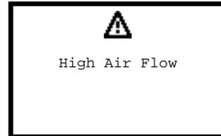
Activated by the differential dirty filter pressure switch (PFS); only causes an alarm signal, without unit operation being affected. Indicates that the air filter needs to be cleaned or replaced.
