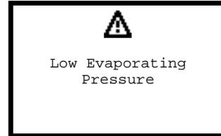
CW units only. Activated by the chilled water air flow pressure switch which signals a lack of water within the hydraulic circuit.
