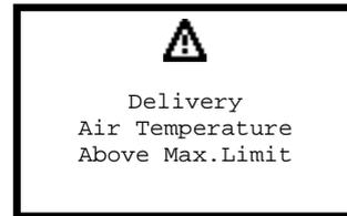
Signal only. This can be delayed during the unit start-up phase (the default delay is 15 minutes).
