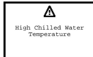
TC units only: causes the changeover from chilled water operation (CW) to direct expansion (DX). It is also displayed when the ambient temperature sensor detects that the limit set has been exceeded for the first time.
