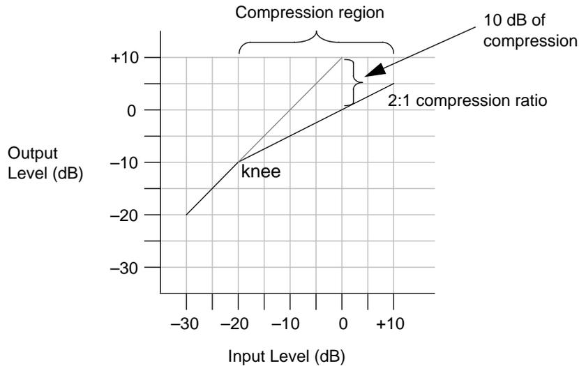
Figure 4. Input and output curve of compressor with 2:1 ratio and -20 dB threshold
