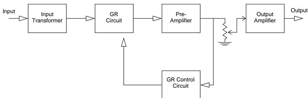
Figure 7. 1176LN signal flow
