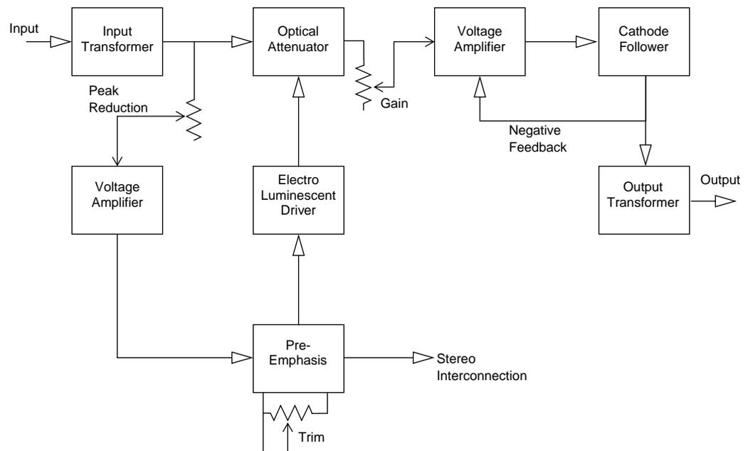
Figure 5. LA-2A signal flow
