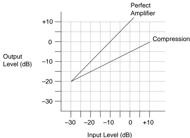
Figure 3. Input and output characteristics of a compressor and perfect amplifier
