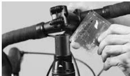
Apply some carbon assembly paste on the steerer tube
