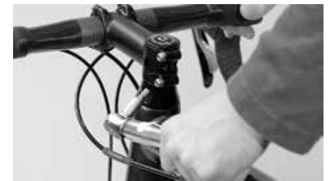
Retighten the stem to the prescribed torque
