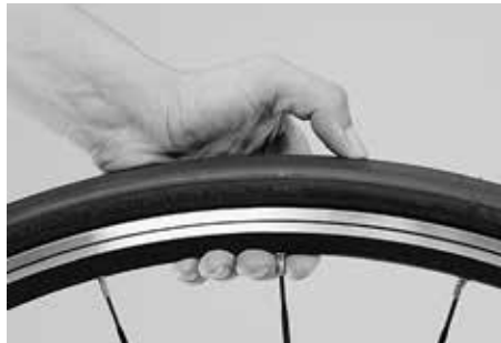
Check the air pressure at regular intervals
