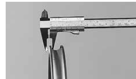
Have the thickness of your rims checked at the latest when you are through your second set of brake pads
