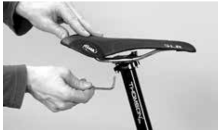
Release both bolts by two to three turns at the most
