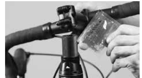
Apply some carbon assembly paste on the steerer tube
