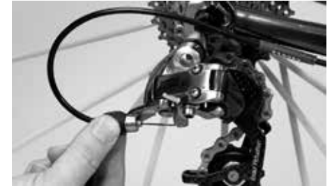
Retightening of the bowden cable at the adjusting bolt of the rear derailleur
