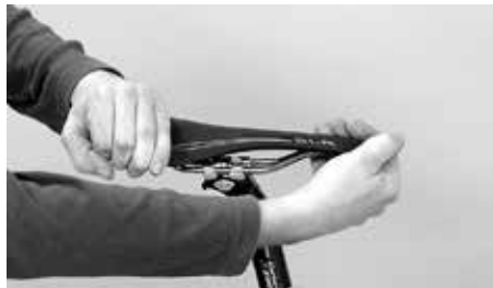
Try twisting the saddle relative to the frame
