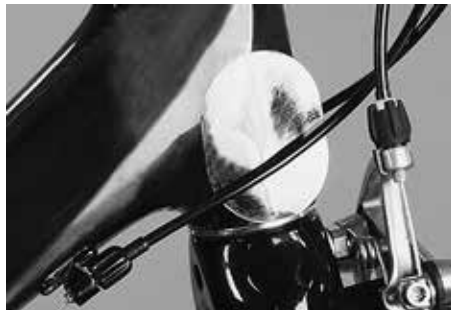
Special pads protect carbon from damage
