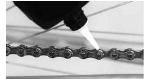
Clean the chain as thoroughly as possible and apply lubricant
