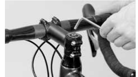
Adjust the bearing play by means of the countersunk adjusting bolt at the top after releasing the clamping bolts on the side
