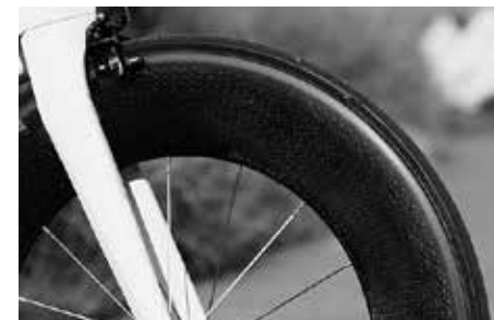
Wheels with carbon rims have a particular brake behaviour
