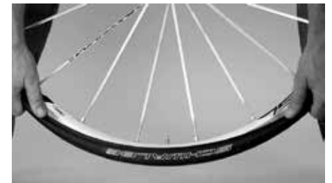
Press the tyre with your hand onto the rim
