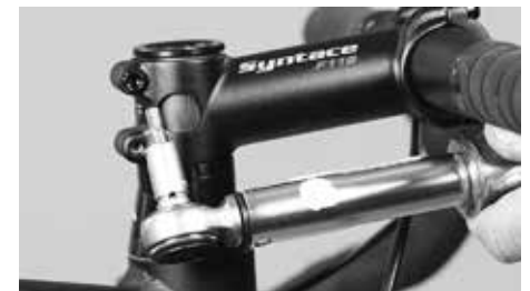
Retighten all bolts of the stem clamp with a torque wrench by observing the correct tightening torques
