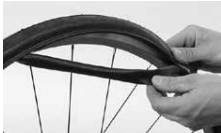
Remove the inner tube from the tyre
