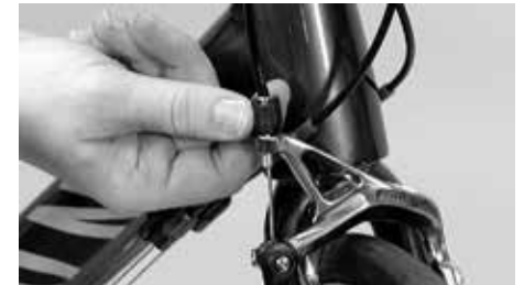
Turn the knurled nut to adjust the necessary brake lever travel
