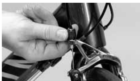
The necessary brake lever travel can be slightly modified by means of the knurled nut
