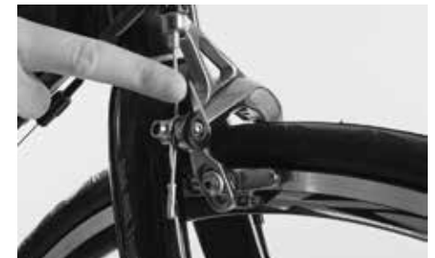
Opening the release lever at the brake
