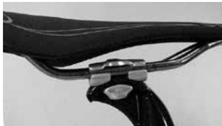
Be sure the saddle rail is clamped within the marked area
