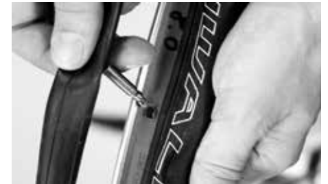
Put the valve into the rim hole
