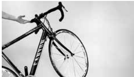
To check the bearing for ease of running, lift the front wheel and move it
