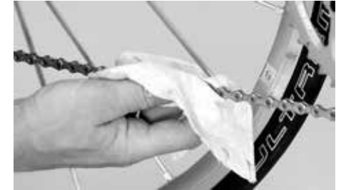
Clean the chain from dirt and oil with a rag
