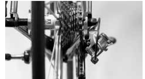
Look from the rear at the rear gear cluster and check whether the pulleys are perfectly aligned with the teeth of the adequate sprocket
