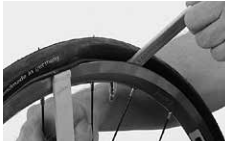
Apply the tyre levers and lift the tyre bead over the rim edge
