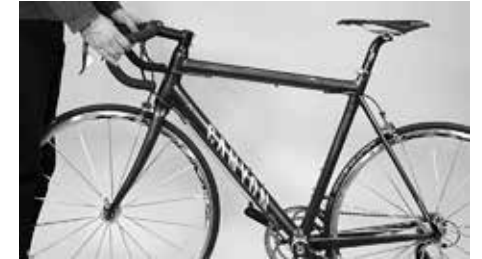
Try twisting the handlebars relative to front wheel and stem
