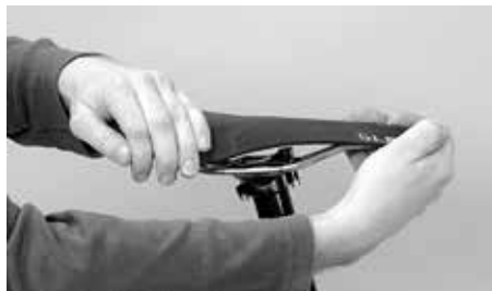
Try twisting the saddle relative to the frame
