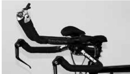
Bar end shifters operate rear and front derailleur
