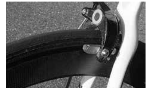
Carbon rims require special brake pads according to the instructions of the wheel manufacturer
