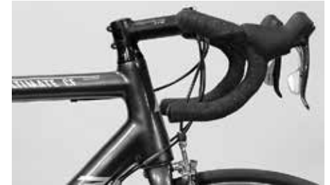
The straight extension below the drops should be parallel to the ground or slant slightly downwards towards the rear
