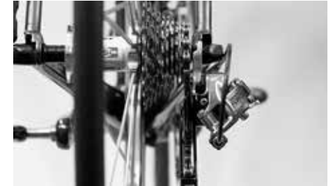
Shift to the smallest sprocket before dismounting the rear wheel
