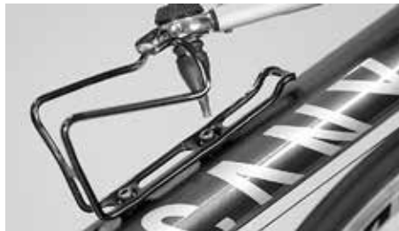
Do not exceed the maximum torque of 4.5 Nm when tightening the bottle cage
