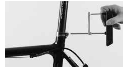
Take care not to overtighten the seat post binder bolt
