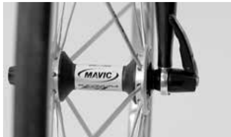
The quick-release lever must be nearly parallel to the wheel and not stick out
