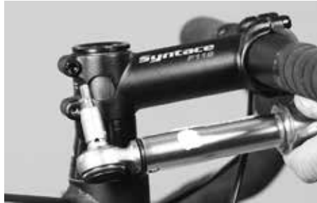
Use a torque wrench to check the stem clamping bolts on the side according to the marked torques
