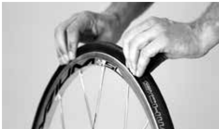
Press the tyre to make sure the tube does not get caught between rim and tyre beads
