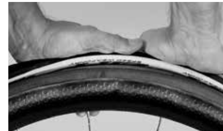
Roll off the tyre until there is a gap
