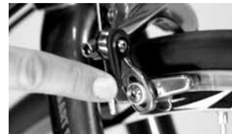
Checking the true running with brake pads
