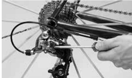
Reduce the swivel range of the rear derailleur with the limit screws
