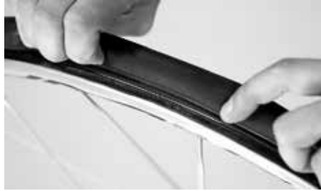
Press the tyre towards the centre of the rim
