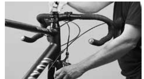
Remount the cap and press it downwards to the fork you keep hold of and retighten the aligned stem to the prescribed tightening torque
