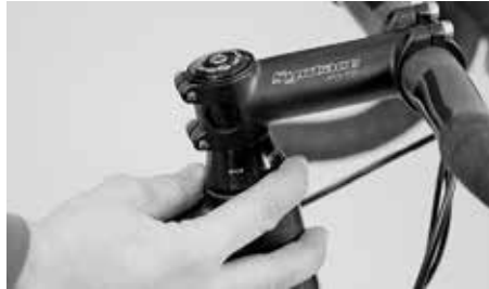
Check the headset for play by placing your fingers around the upper head cup and by moving your Canyon back and forth with actuated brake lever
