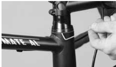
Turn back the counted rotations of the headset adjusting device
