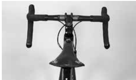
Make sure the saddle is not twisted using the top tube as a reference
