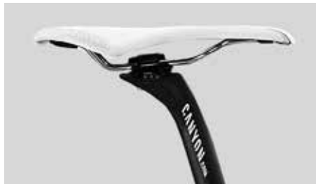
Do avoid a rearward tilt of the saddle
