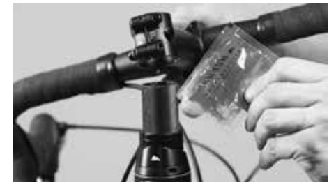
Apply some carbon assembly paste on fork tube or handlebars, if necessary
