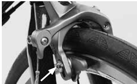
To adjust the height of the brake pads tighten the bolt to the prescribed torque
