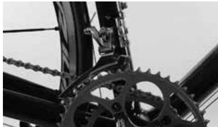
Adjusting the swivel range of the front derailleur
