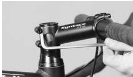
Release the bolts on the side of the stem
