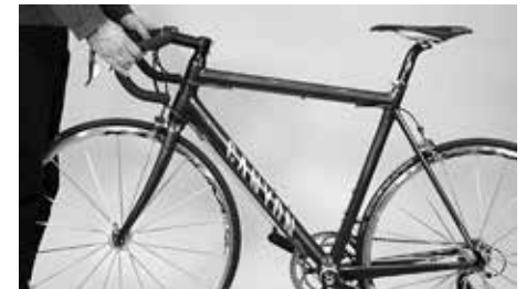
Try twisting the handlebars relative to the front wheel
