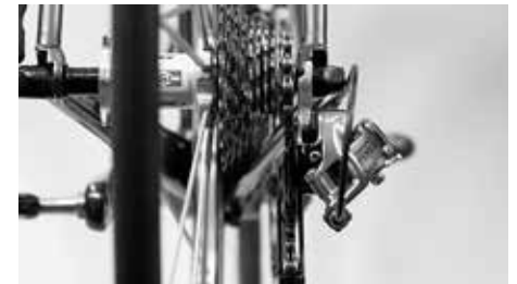
Verify that the chain still runs on the chainring and sprockets
