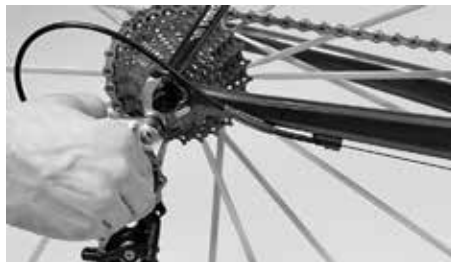
Check whether the rear derailleur remains clear of the spokes
