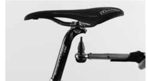
Tighten both bolts evenly and alternately without exceeding the permissible maximum torque
