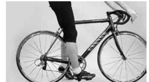
The leg must be fully stretched with the heel on the pedal at its lowest point
