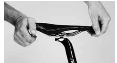
Check the firm seat of the retightened saddle
