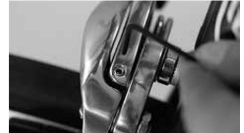
Screw this small bolt until the clearance between brake pad and rim is the same on either side
