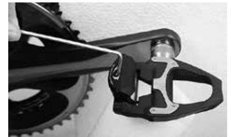
Adjusting the releasing force of the pedal
