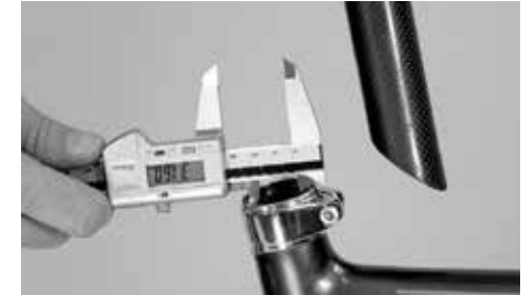
Make sure the seat post matches accurately the frame
