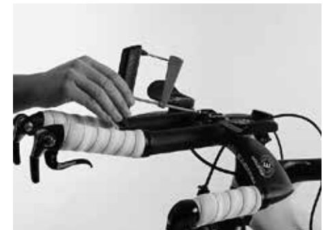
Mounting the handlebars with the Canyon torque wrench
