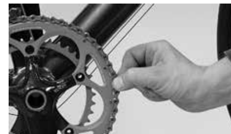
Check condition of chain
