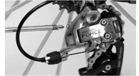
To adjust the clearance between pulley cage and sprocket, turn the bolt located at the front side of the drop-out
