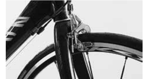
Check of wheel trueness with brake pads
