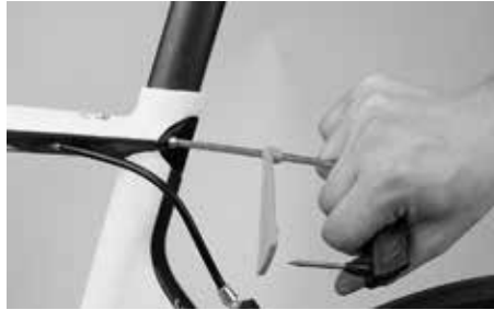
Tighten both bolts by using a torque wrench
