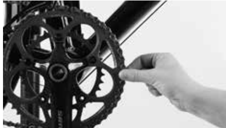
Check condition of chain
