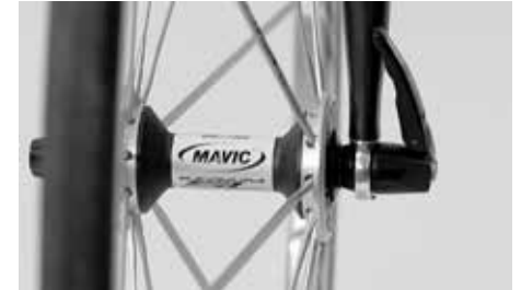
Check the reliable clamping of both wheels between the drop-outs
