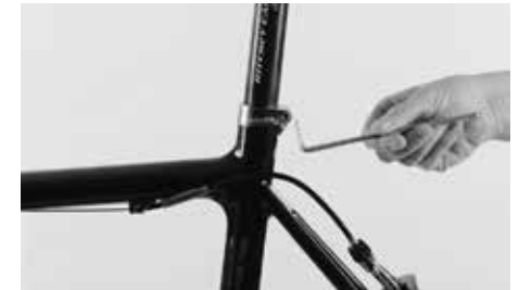
To adjust the saddle height loosen the seat post binder bolt
