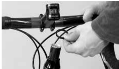
Remove the spacers under the stem and place them above the stem
