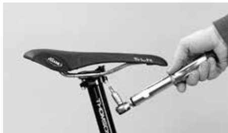
Retighten the bolts evenly and alternately to the prescribed torque
