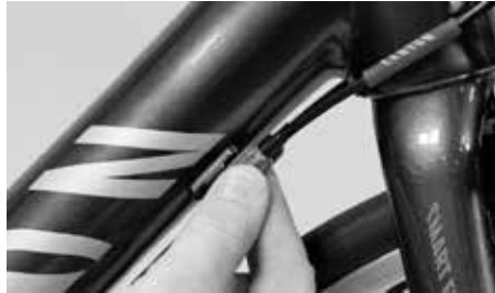
Retightening of the bowden cable at the adjusting bolt on the frame
