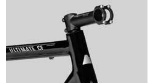
Fully mounted and adjusted headset with stem and fork
