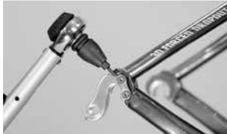
Do not exceed the maximum torque of 1.5 Nm when replacing the replaceable derailleur hanger
