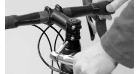
Retighten the clamping bolts located on the side of the stem by using an Allen key
