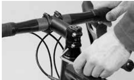
Release the bolts on the side of the stem
