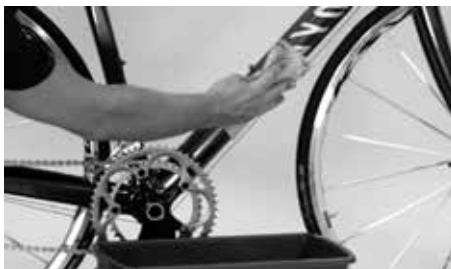
Cleaning the Canyon with rag and water
