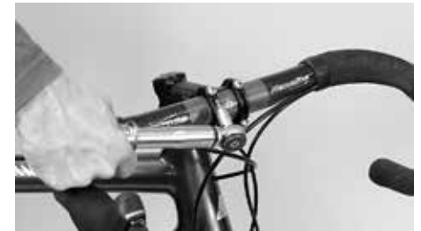
Retighten the bolts to the prescribed torque
