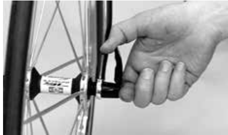
Open the quick-release lever
