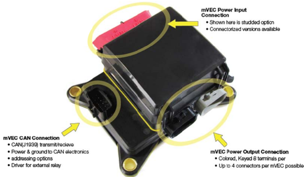
Figure 7. Connector locations
