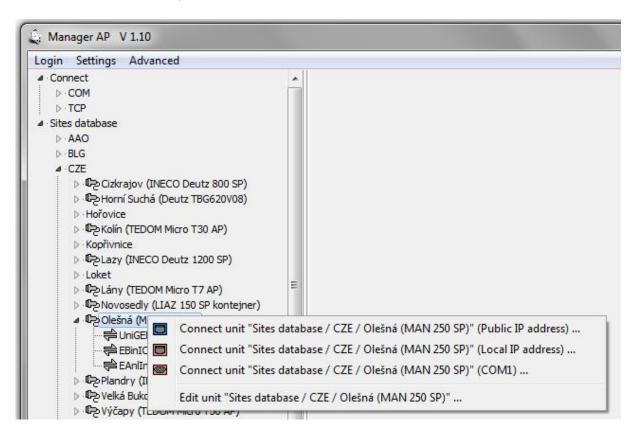
Use left mouse button to mark the unit from the database (number of COM or IP address of the connection) to which you want to connect.
