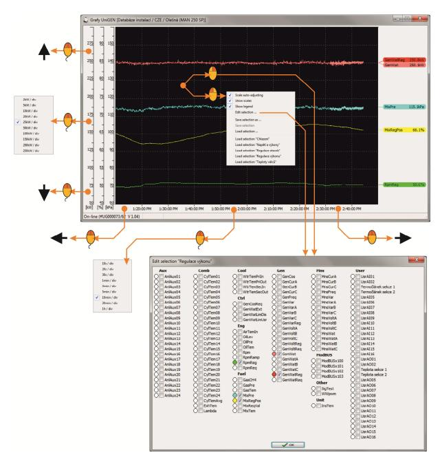
By clicking in the area around the middle part of the scale you can select the range (value per division) both on the Y axis and the time axis.
