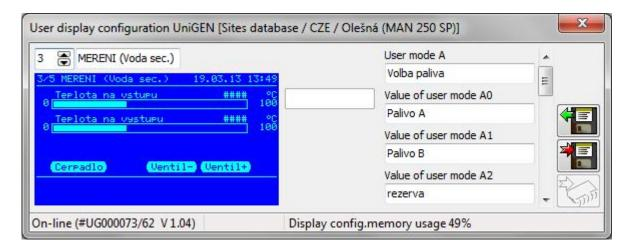
It is also possible to define two user items in the menu "Service" (User Mode A and B) and define four different submenu options for either of them. In functions it is possible to use in any way signals "User mode A0 (A1)", and "User mode B0 (B1)". In each of the modes these two signals represent by their binary combinations one of the four items selected in the menu:
