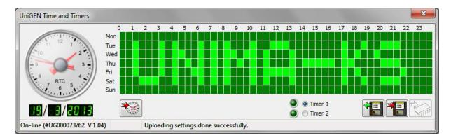
Using your mouth you can define the weekly schedules in half-hour intervals. If the field is bright, the signal of the timer 1 (2) "Timer 1 (2)" is active in the given half-hour if the field is dark, the signal is inactive. The signal is activated with the left mouse button and deactivated by the right mouse button.
