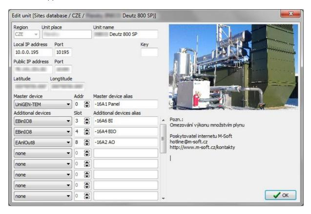
The Program will add to the form the control system found and other additional equipment. After adding other available data (unit name, IP address, etc.) and pressing OK, the unit will be stored in the database. It is important to fill in the "Region" and "Installation Location", these data cannot be edited later and they specify the directory in which all subsequent unit data will be stored (see Directory Syntax in the previous section).
