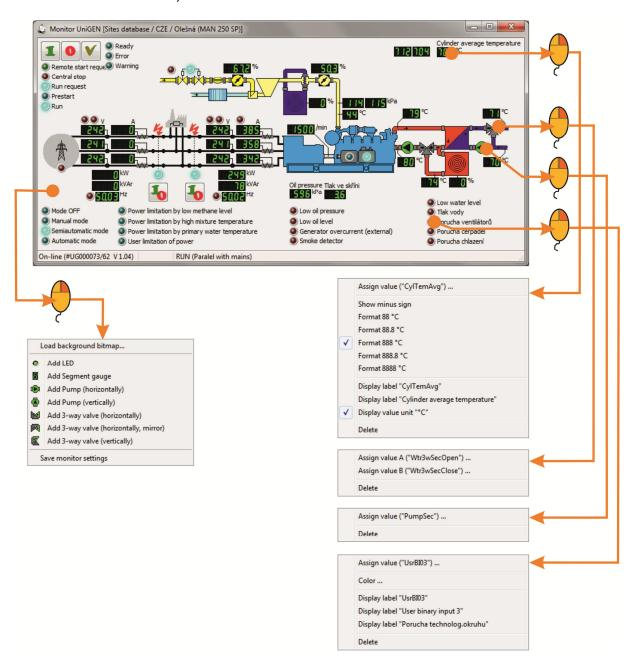
This window can be customized in the installation (if the user is logged with the right to configure the monitor, and if you are connected to the unit from the installation database). By right-clicking on the free space of the window a menu will pop up to add an object to the monitor:
