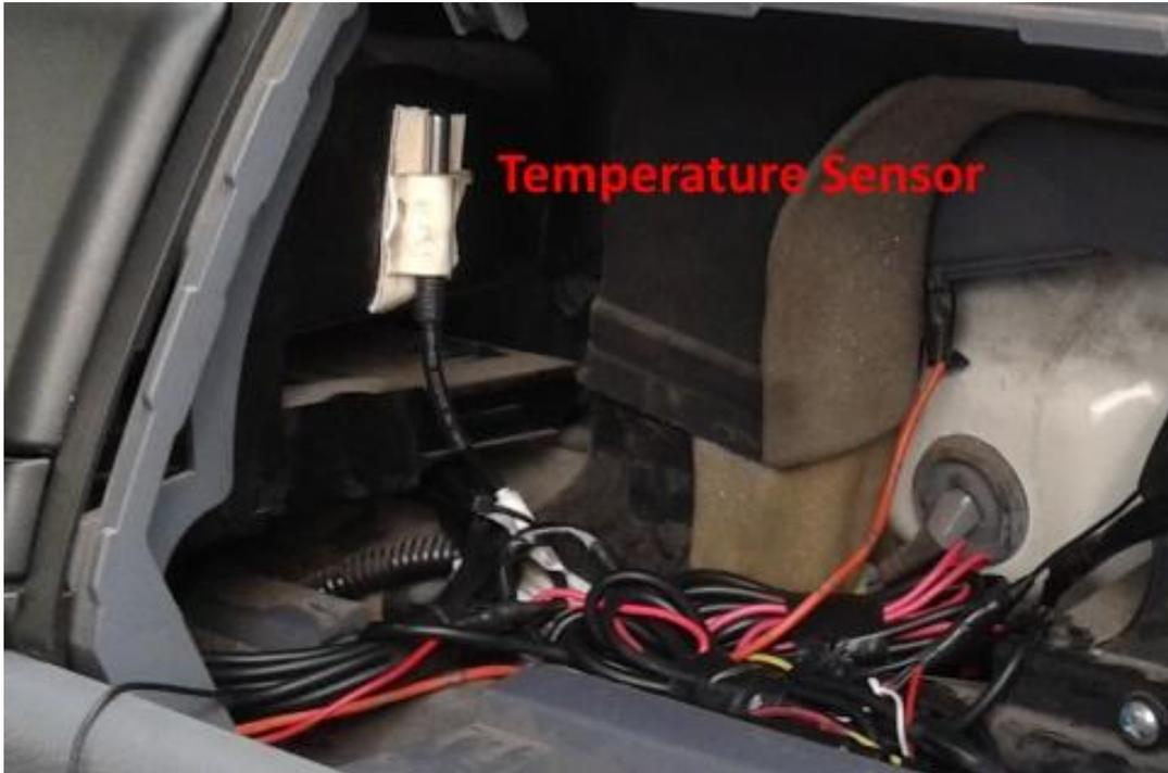
Temperature Sensor installed under dashboard
