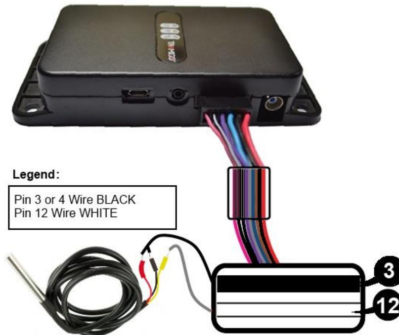
Temperature Sensor connected to T23 Fleet
