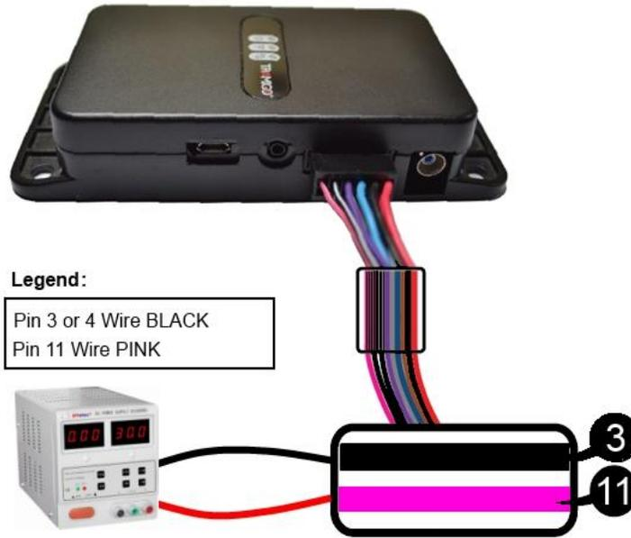
Voltage source connected to T23 Fleet
