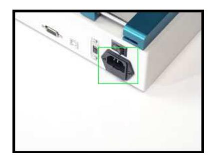
Step 2: Remove the fuse holder from the power plug. There is a small indentation on the bottom edge of the power plug. A small coin or screw driver may be needed to remove the fuse holder from the pump.
