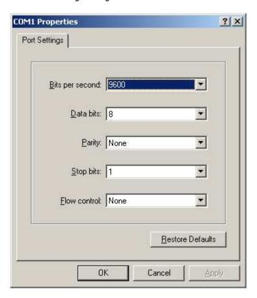
After you press OK you will come to a blank window with a blinking cursor. You can type in protocols here to test communication or to run the pump from a remote computer. Connect the pump to the PC. Type in "help" and then press enter to get a complete list of protocols available to the pump.
