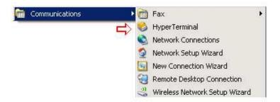
Click HyperTerminal to start the program. Configure the COM port with the following settings.
