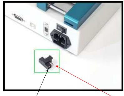
There are 2 fuses in the fuse holder. The exposed fuse in the back is the fuse that is being currently used. In the event of a power surge this fuse will be the broken fuse. Step 4: Remove the broken fuse from the active slot in the holder. Most of the time and broken fuse will be visible to the naked eye.
