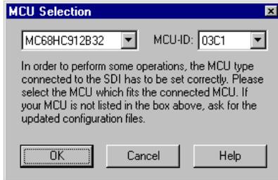
This dialog box contains drop-list combo controls for the name and MCU-ID of the currently selected MCU. Use these controls to make any appropriate changes.
