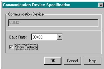
**Maximum Baud Rate** The maximum baud rate depends on the speed and interrupt load of the host computer. For slow notebook computers, or for computers running in a network, the maximum baud rate may be as low as 19200. A buffered I/O card may allow the maximum rate of 57600 for any host computer. The default value is 9600.
