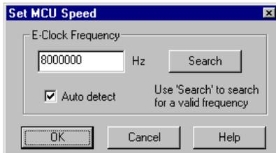
This dialog box shows the E-clock frequency that the MCU is to use, typically half the oscillator frequency. The SDI must know the E-clock frequency for proper BDM communication.
