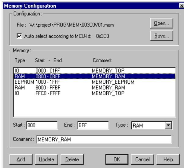
This dialog box shows the default memory configuration for the MCU being used. Check the *Auto select* box to have the system load this setup automatically. The system reads memory-layout information from the specific MCU personality file. The personality-file decomposition is: 00nnnVvv.MEM – nnn is the 3-digit hexadecimal representation of the MCUid, and vv is the version number.
