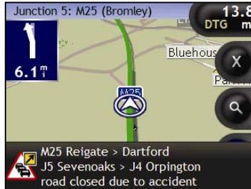
A message will display at the bottom of the screen used to view your route. This details the road name, the section of road affected and the type of Event that has occurred. The message remains on screen for 8 seconds and is added to the *Event List*.
