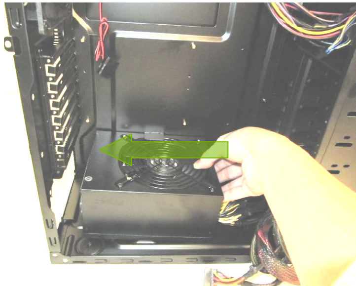
PSU resting on the standard PSU mount.
