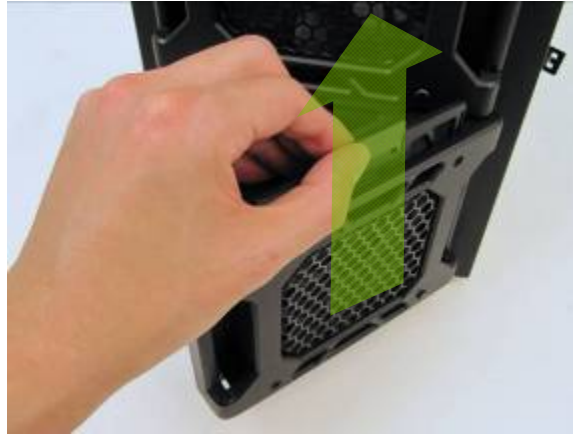
Removing the washable air filter. Note the filter tabs.
