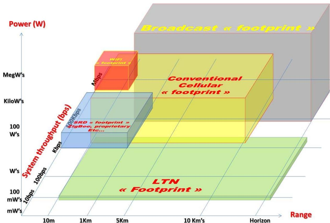
Figure 1: Energy & throughput range comparison
