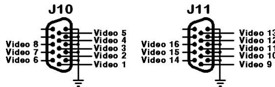
Figure 5. D-Sub 15pin video input connectors
