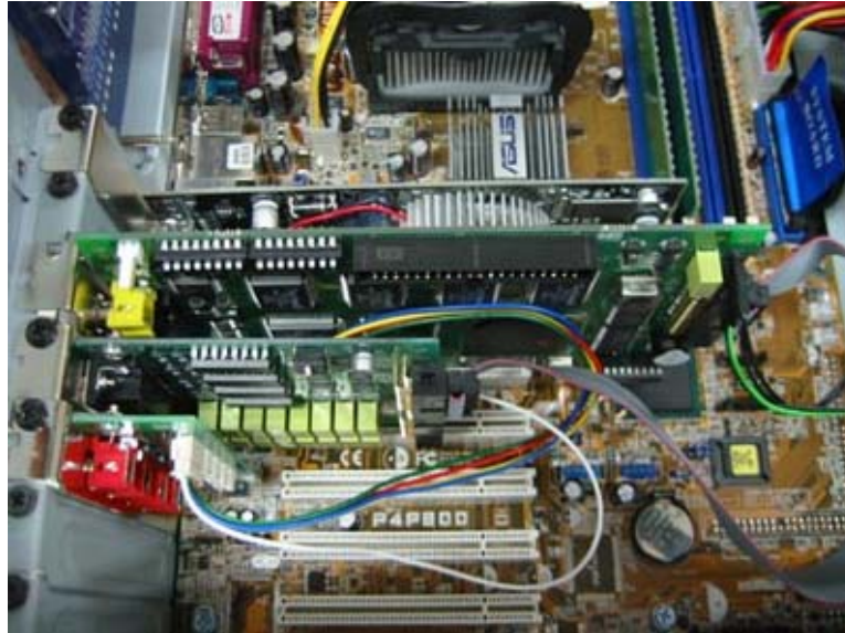
<16120R, AudExt2 and ConExt1616 Inserted into PCI Slot>
