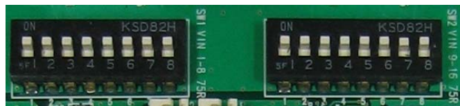
Figure 4. DIP switch (75 Ω video terminal resistor)
