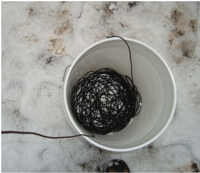
Capture recovered line in a bucket, and it won't tangle when fed out again.
