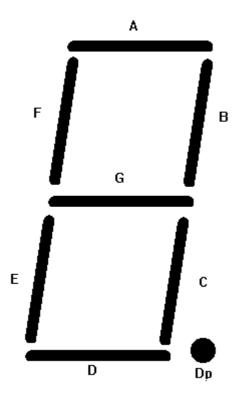
**Example 6** - to send the character S to digit 5. First calculate which segments are on and which are off.
