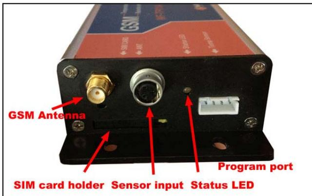
On the side panel of Wafer GSM-TP, it has GSM Antenna Connector, Sensor Input Connector, SIM Card holder, Program Adapter.
