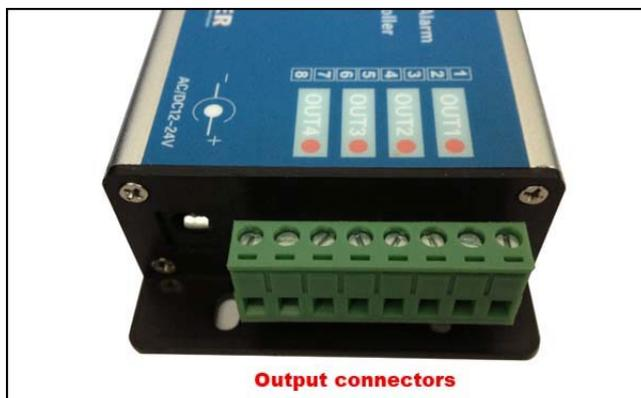
GSM-TP also comes with additional 4 Outputs. The outputs can be controlled through the phone calling or the SMS command.
