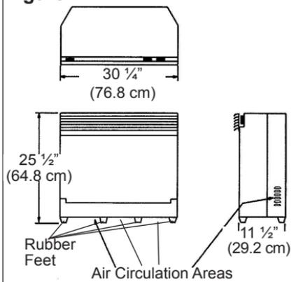
**restrict air circulation.** If installing the fireplace in a carpeted area, place a one-piece, solid, flat surface under the fireplace insert. Ensure that all four of the insert's feet rest securely on this surface.
