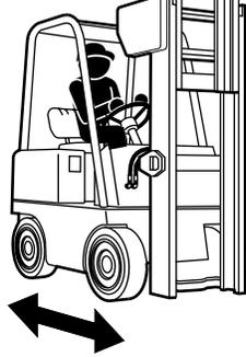
Limit truck movement with raised load.
