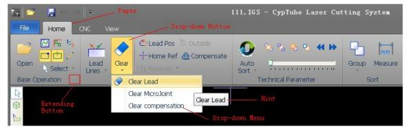
The whole toolbar is divided into four "pages", which can be selected by the four menus "Start", "Drawing", "Numerical control" and "View". When selecting text and other special objects, the pages related to the selected contents will appear. Furthermore, the page "Being Processed" will appear
