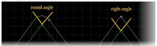
In the figure the green is the original, the white is the compensated track, and the light yellow is the vertical lines drawn from the corner. From the figure you can find that the cutting edges can coincide with the original after both sides of the vertical lines are compensated, while the corner needs transition. Usually round angle transition can ensure that the cutting edges can still coincide with the original and run more smoothly during transition.
