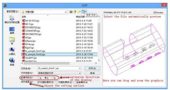
Note:Please make sure the extension direction of the drawing you opened is same as the original extension direction of the drawing. And it's better to create fillet surface when drawing the tube. The cutting outline can be identified automatically, and the gray lines are auxiliary lines which don't need to be processed.
