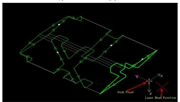
If the "Laser Head Position" shown by the red cross cursor does not match the actual laser head position of the machine, please check whether the position of the machine origin is correct, and it can be corrected through "Numerical Control"—"Go Origin". After previewing, if you find that the graphics are outside the machine breadth wholly or partially, it means that it may exceed the range of travel during processing.
