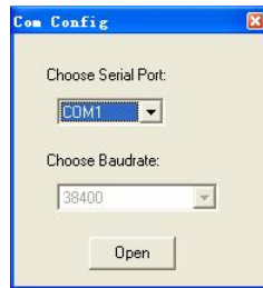
Figure 21: RS232 communication configuration window
