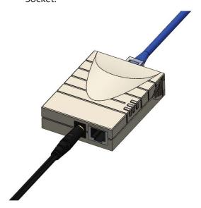
Optional: If you wish to connect to the HOD45B using an Ethernet cable from a computer, connect an Ethernet cable to the port labeled "LAN" and plug the other end into your computer. Skip to Step 3.
