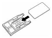
3 Insert the USIM/SIM card slot into E220.
