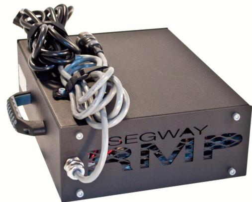
Figure 48: External Power Supply
