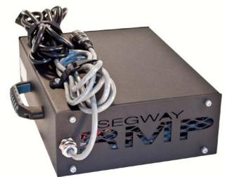
Figure 4: External Power Supply
