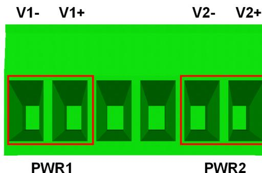
Insert the positive and negative wires into the V+ and V- contacts on the terminal block connector.
