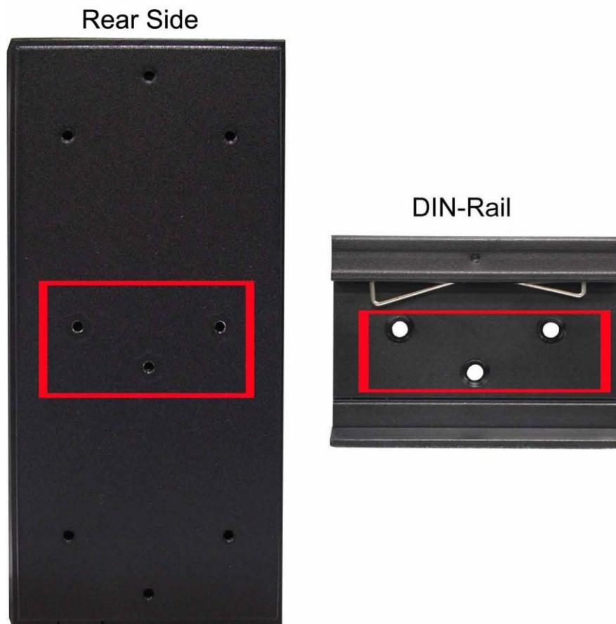
**Step 1:** Use the screws to screw on the DIN-Rail on the industrial switch.
