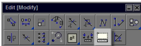
For instance if you have drawn a rectangle DynaSCAPE Design will calculate all the lengths of the lines that make up the rectangle and give you an overall length.
