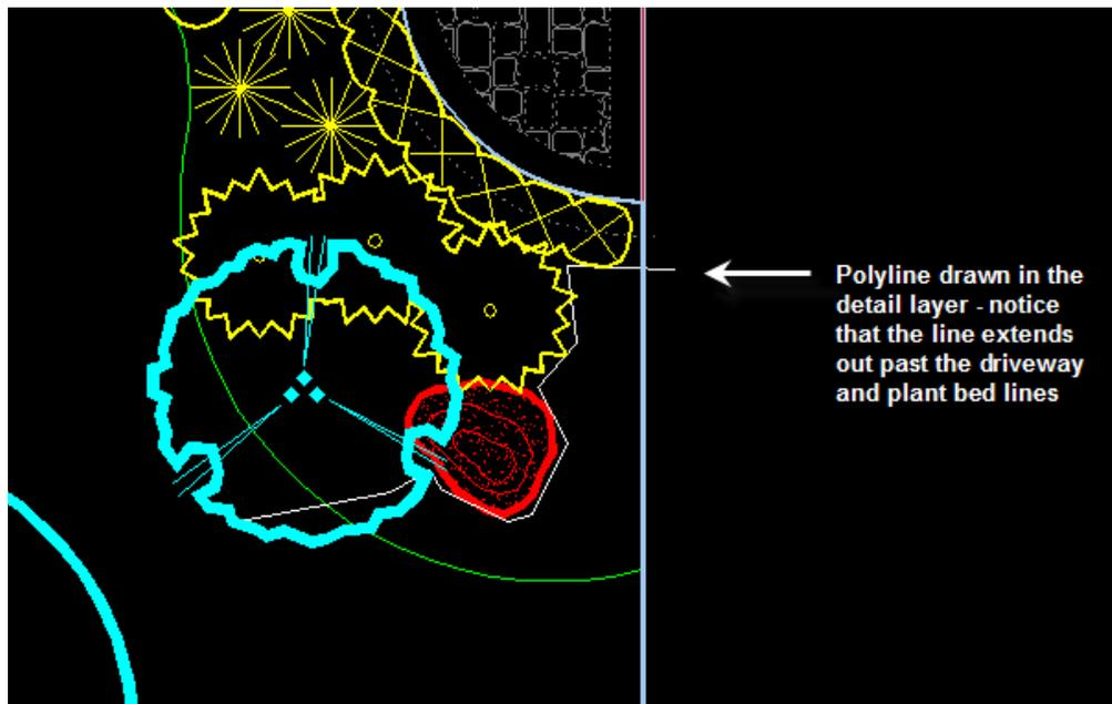
4. To insert the pattern into this area first select the **Annuals** layer and then right-click the 'Section a Bounded Area by Selecting a Contained Location' tool to open its hidden modifier. (You may need to uncover the nested Section tools if they are not already visible.)
