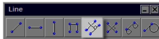
This tool allows you to draw a line parallel to an existing line on the drawing at a set distance away (offset). A modifier panel allows for the length of the parallel line and the distance it is set from the existing line to be set, ensuring accuracy.
