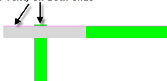
If the first line of the building is too short to trim to, use the 'grips' to extend it first. To do this, first press [Esc] and then click on the building line to reveal the grips. Click on the end grip and move it past the second line you drew and left-click, remembering to use your constraints to keep the line straight. You will need to extend both the Building line and the Title
