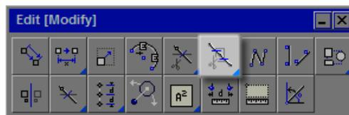
This is a two-step process: Step one is to select the lines to be extended, while step two is to select the line to extend them to.
