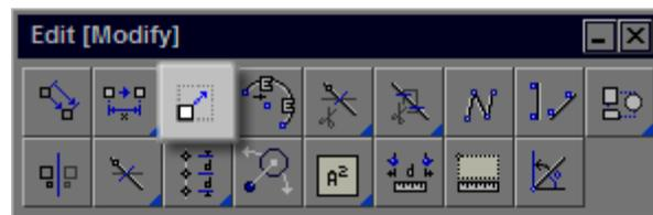
A scale tool exists in DynaSCAPE Design that allows for objects to be resized within the drawing. By applying a scale factor to an object or group of objects, a drawing (such as an imported AutoCAD file— see Chapter 9 for more information) or parts of a drawing (such as a deck area in order to create a more detailed plan off the main drawing area) can be made larger.
