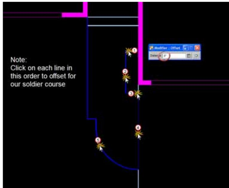
2. The last two lines to offset have to be done separately because one of the lines are part of the house outline and therefore extends above and below the area in which the line is needed, while the other is the step line. If you had attempted to offset these lines along with the other lines, the offset
