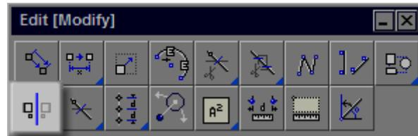
The mirror tool allows you to mirror objects on the drawing. This is an excellent tool for formal gardens or symmetrical details such as screens and arbors—saving time from redrawing the elements twice.
