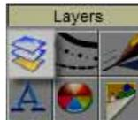
Layers (covered in Chapter 5) are like transparent sheets of paper stacked one on top of another: they allow you to give the same attributes to like entities. For example, all rocks can be drawn with the same color, line weight and line style, and this layer can be turned on or off—just like putting on or taking off a transparent sheet of paper with all the rocks drawn on it—to keep your drawing area uncluttered, even while working on complex drawings.
