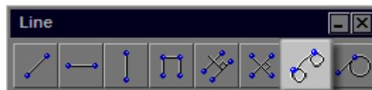
This tool allows you to draw a line tangent to two circles and/or arcs. This tool will only work with arcs and circles and will not recognize polylines unless they have previously been exploded.
