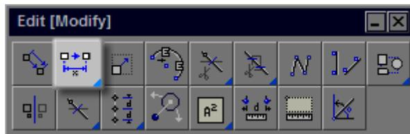
The offset tool allows you to set a distance to move items a set distance away. Basic entities such as lines, polylines, circles and rectangles can be offset so that the new entity is parallel to the existing entity.
