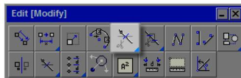
11. The last part of the walkway that needs to be drafted is the step at the stoop. This is done simply by offsetting the stoop line 1'. Using the Offset
