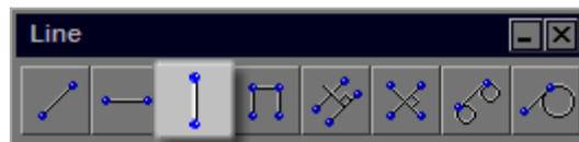
This tool allows you to insert a true vertical line between two points. Using this tool there is no concern for constraints.
