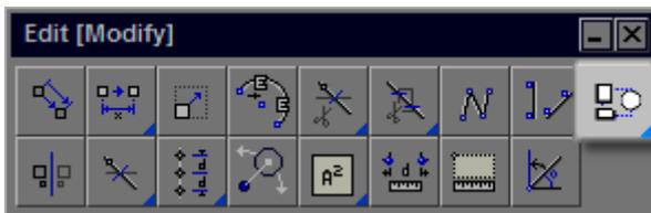
The explode tool in DynaSCAPE allows objects to be broken into individual pieces of geometry. Items such as polylines can be broken into individual lines and arcs. Rectangles can be broken into lines and figures can be broken down into the entities that were used to create the figure.
