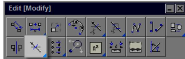
The break tools allows for a line or object to be taken and broken into separate the selection pieces. One break tool is visible in the Edit toolbox however there are a number of additional tools nested underneath.
