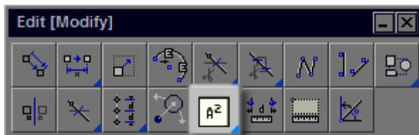
In the **Edit** toolbox in DynaSCAPE there is only one area calculation tool visible. However, there are three area calculation tools available. Two other area calculation tools are *nested* beneath the visible tool—giving you more calculating options. These tools will allow you to calculate the total area measurement within a location.
