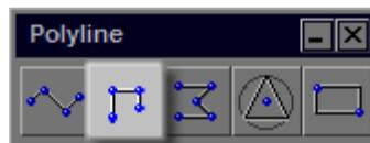
This tool would be used when tracing a lot plan where the building does not sit square on the screen. Using this tool will ensure that all the lines of the building will be either parallel or perpendicular to each other.
