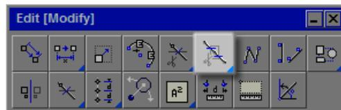
Now you need to trim the excess lines not needed. Select the **Trim (clip) lines to closest intersection** tool and left-click on the two horizontal lines just drawn (the offsets of the stoop line) and then right-click.
