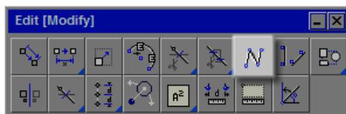
Right-click to end the process. This is now one totally enclosed area which can be selected, moved and filled in as one entity.
