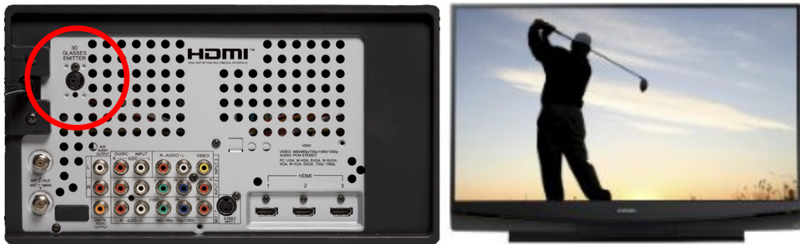
Figure 2: Mitsubishi 3D DLP TV with a 3D Emitter port in the back (left) and alternating frame 3D image in the front (right) that match the timing described here. The emitter will work out-of-the box for this case with no performance tuning.
