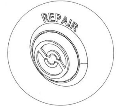
**Note:** Discs can be repaired an unlimited amount of times. However, never run a disc two times consecutively without letting the disc cool to room temperature after each repair cycle.
