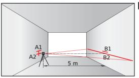
Then place the instrument at the same elevation as close as possible to wall A and again mark the horizontal laser line or the laser dot on wall A (-> A2). Rotate the instrument by 180° again and mark the laser on wall B (-> B2). Measure the distances of the marked points A1-A2 and B1-B2. Calculate the difference of the two measurements. If the difference does not exceed 2 mm, then the CLL 11/PLL 11 is within tolerance.  $| (A1 - A2) - (B1 - B2) | \leq 2 mm$
