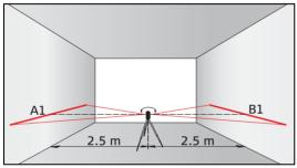
Set the instrument on a tripod half-way between two walls (A+B) that are approx. 5 m apart.
