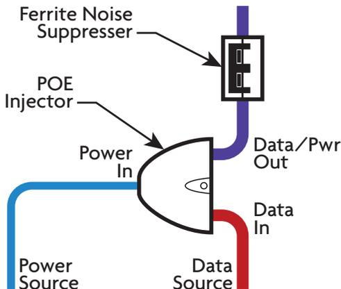
*The POE Injector Sends Power and Signal Over One Ethernet Cable*
