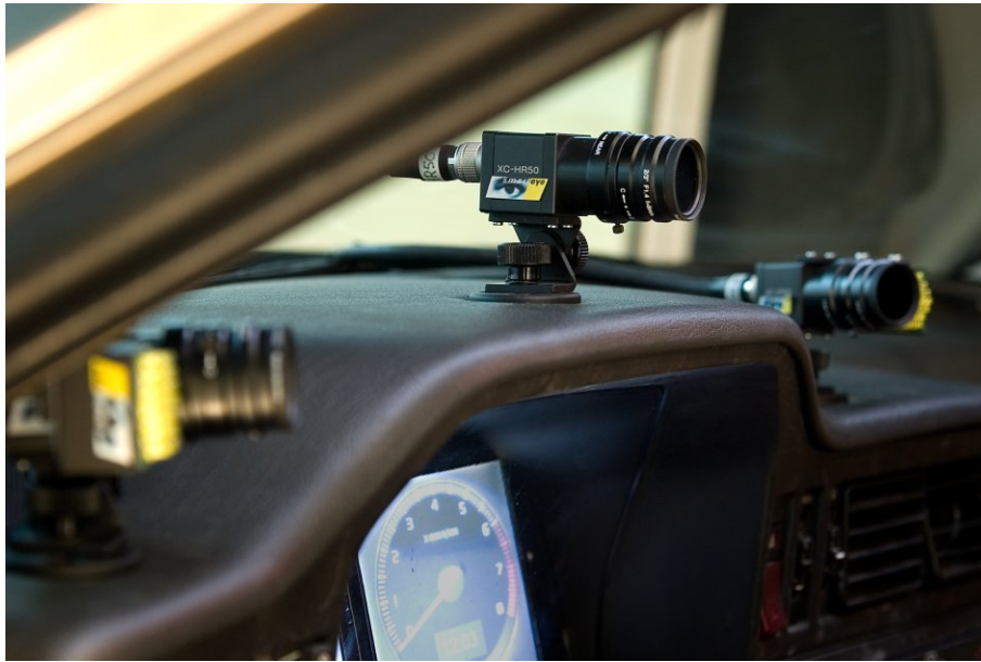
Figure 3.1: Smart Eye cameras in VTI Simulator III
