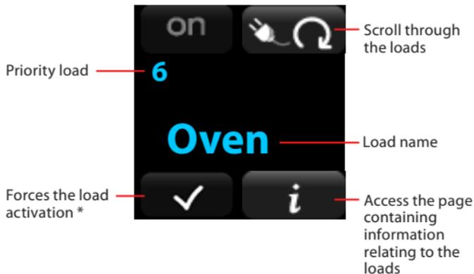
\* When performing this action, the load is no longer controlled by the load management central unit.
