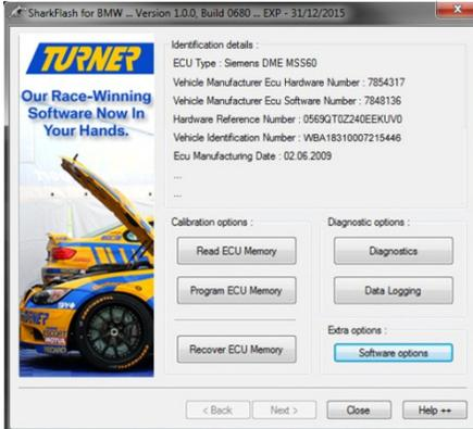
The first action is to check for existing fault codes in your ECU. This is also a communications test between your car and the SharkInjector tool.
