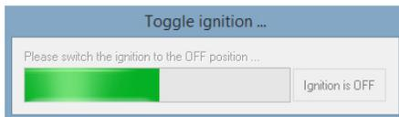
After the update is complete turn off the ignition via the Start/Stop button. Click the [Ignition is OFF] button on the screen. When the green status bar is done counting down your ECU is now ready for the Performance Software install.
