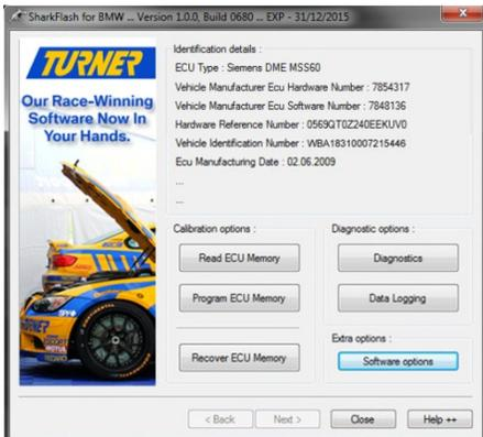
This is the main SharkInjector functions menu. At the top is the specific info for your car's ECU. At the bottom are the buttons for running the various SharkInjector functions –
