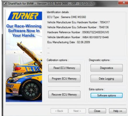
We require you to install an updated Turner version of stock software before the tuned file can be loaded. This is a new Base file similar to the factory “240E” file. This is mandatory and you must ensure the Turner 240E base software is installed before continuing with the tuned software install.
