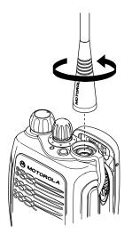
Turn the antenna counterclockwise to remove it.
