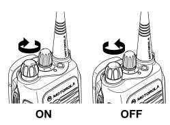
Turn the radio on by rotating the volume control clockwise. The radio goes through a power-up self check and, if it passes the check, a good-power-up, high-pitched tone sounds to indicate that the radio has passed the self check.
