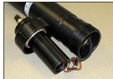
**DO NOT** impact the threads on the VR2C or they will dent and prevent the VR2C case from closing. See the Trouble Shooting section of the Appendix for tips on thread care.
