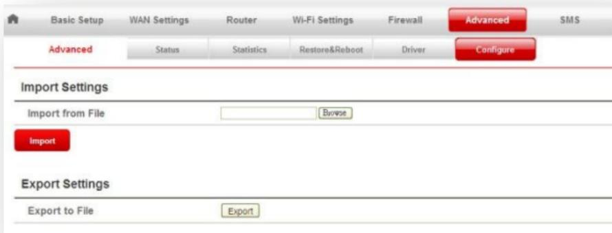
The **Configure** page allows you to export configuration settings of the device to your computer or import configuration settings from your computer to the device.
