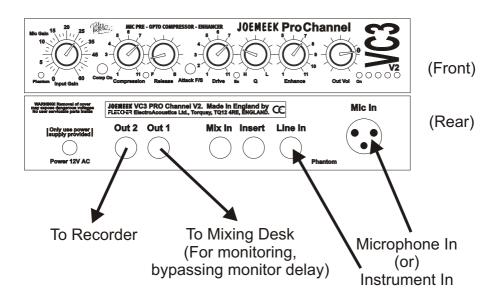
The mix input may be used to add additional sources at the performance, and the insert point may be used to add effects by diverting the line level signal through and external processor (i.e. reverb unit or amp simulator).
