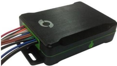
Note: The device side with the Meitrack logo faces upwards to get better GPS signal.
