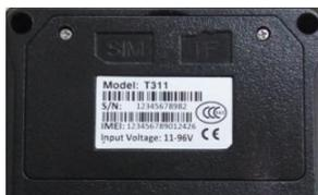
Turn off the device. With the back panel facing you, use the mini screwdriver to remove the two screws to release the back cover. Then lift up the back cover from the notch at the bottom of the device.
