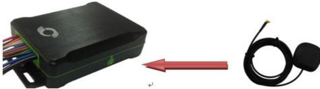
Connect the GPS antenna to the GPS port on the side panel of the tracker. It is recommended that the antenna should face up to the sky and the antenna side with words should face downwards. Secure the antenna by using double sided tapes.
