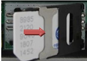
Gently push the SIM card into the slot until you hear a click with the gold-plated contacts facing down.
