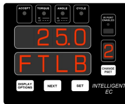
Example: PSET #2, Torque Control Strategy, 25 ft-lb Target
