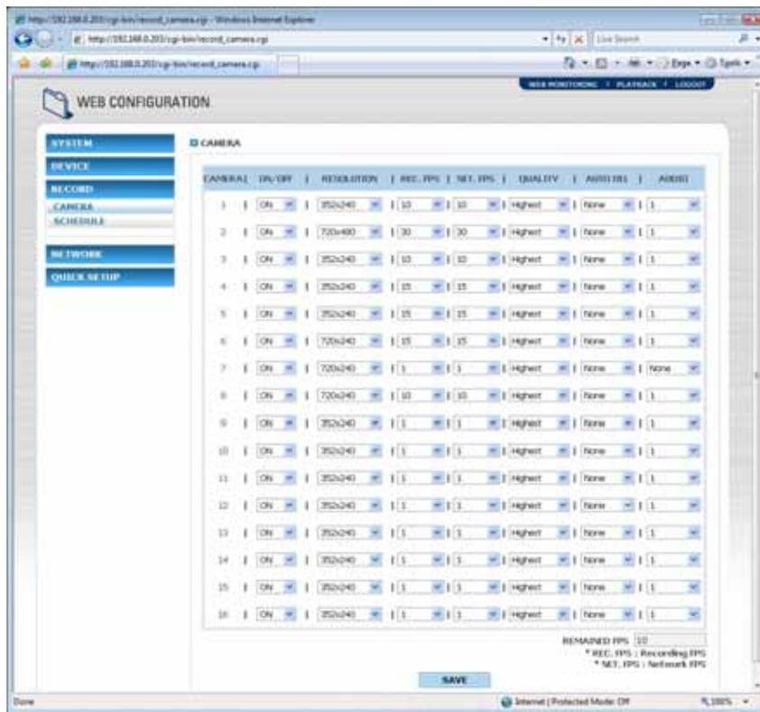
You can adjust frame per second (FPS) and resolution of each camera, based on the REMAINED FPS left.
