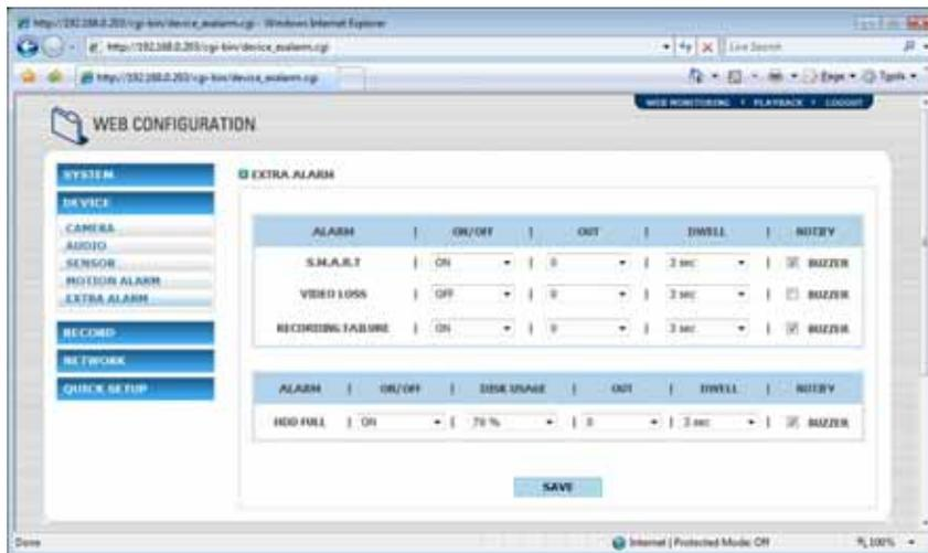
S.M.A.R.T : setup alarm for HDD health
