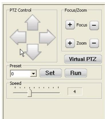
PTZ Control : Camera can be moved up, down, left and right
