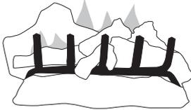
Figure 12 - Correct Burner Flame Pattern
