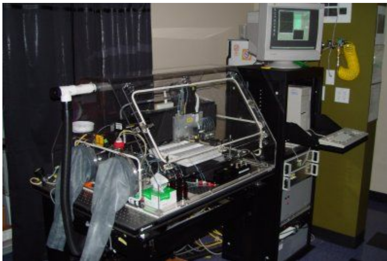
Figure 1. We recommend placing the electronics rack to the right of the table. This allows the operator to access the front door and the gloves on the left.
