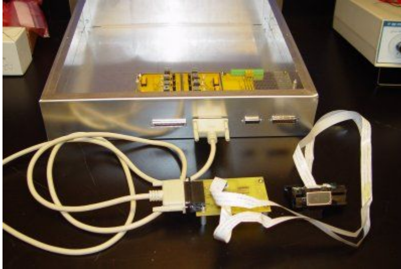
Figure 7. View of the 1804 board installed in a 19" rack, before installation of the power supply, power connectors, switch, and front panel diodes. The 120VAC receptacle, the power supplies, and the front panel parts are not yet installed.
