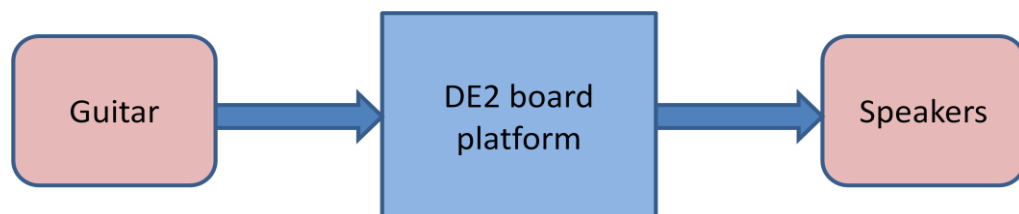
Figure 4.1: Block diagram for the guitar effect sound system
