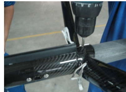
Tap 4mm hole with M5 tap
