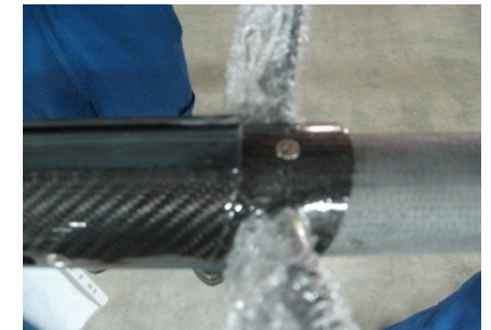
Fasten CSK M5x12mm fastener
