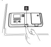
Insert detergent: Tablet / powder / liquid into the big chamber.
