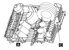
Cutlery basket - half (B): can be placed in the upper rack when the "Half load/ Multizone" is selected. The Grid (E) should be removed.
