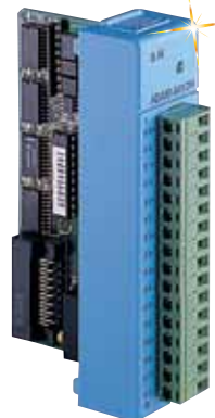
ADAM-5017H, 8-channel high speed analog input, shown smaller than actual size.
