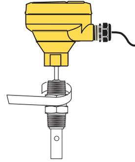
The preferred installation for in-line applications directs flow straight into the electrode. This configuration reduces the probability of entrapped air bubbles, and provides the best continuous sampling of the fluid content.
