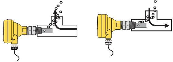
If the electrode is mounted vertically in a tee, do not recess the electrode orifices inside the tee. Mounting upside down may help prevent air entrapment.
