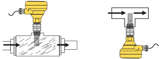
Use the 2850-6X models for in-line installations where the electronics must be separated from the electrode. Conductivity electrodes with sanitary flange fittings must be installed using this option.
