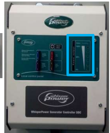
Figure 3: Remote and DDC box load indication
