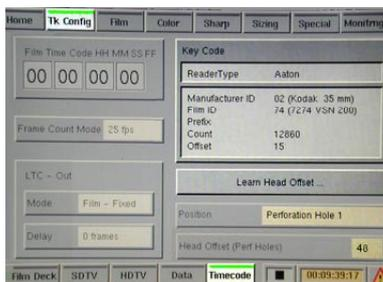
Keycode data being 3 frame delayed, another delay must be added by the GCP-controller (e.g. 15 - 3 = 12 frames = 48 perfs). Please carefully read the «Learn Head Offset» paragraph 5.9.4 page 61 of the Spirit
