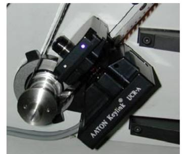
Note: the UCR-A head is mounted on a U2 two position carrier which allows to downward rotate the head to leave room for opening the mirror holder when cleaning the CRT face plate (see pict. end of this section).
