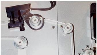
**\* CTM Dixi-2** The 35>16  $\Delta=0\text{mm}$ , Keycode operator side. UCR-B head w/ S1 carrier clamped to the upper roller.
