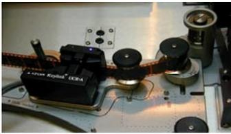
Note the middle position of the base plate for the Aaton head.
