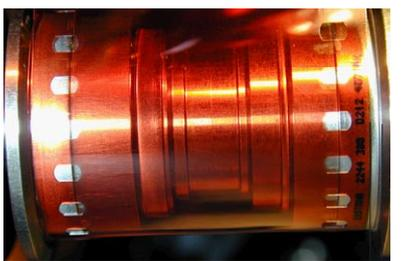
makes the film flush to the deck-side flange. If this is not the case, loose the two screws of the deck shaft holder, move the shaft up (e.g. by a few tenth of a millimeter) until the film runs in permanent contact with the deck-side flange.
