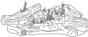
Figure 39 - Correct Flame Pattern with Control Knob Set to High Flame.
