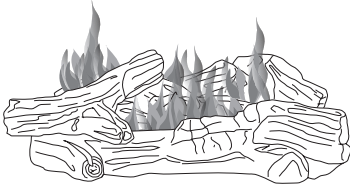
Figure 40 - Incorrect Flame Pattern with Control Knob Set to High Flame
