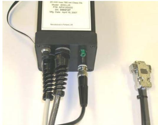
**Figure 16 - Cabling of AR4000 with 200 KHz capability**
